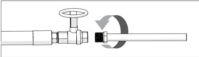
5. Connect female quick-connect fitting to output side of foam unit discharge valve. Female quick-connect fitting has ½ in. male NPT threads. **Only install quick-connect fittings on output side of foam unit discharge valve, as shown in the Installation Instructions. Do not install in any other configuration.**
