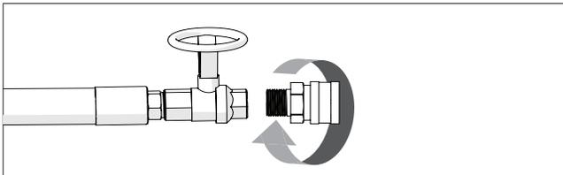
6. Connect male quick-connect fitting to foam unit wand. Male quick-connect fitting has ½ in. female NPT threads.
